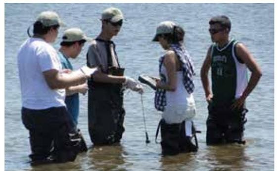
*Students using a high tech multi-parameter water analyzer*
