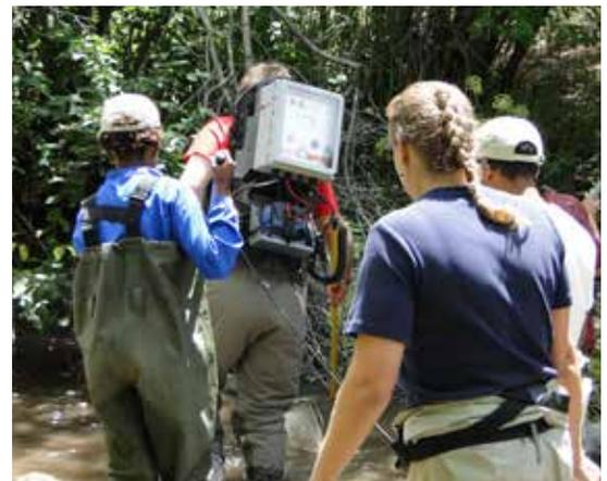
*Properly supervised, students using the Electro-shock fish survey backpack unit*
