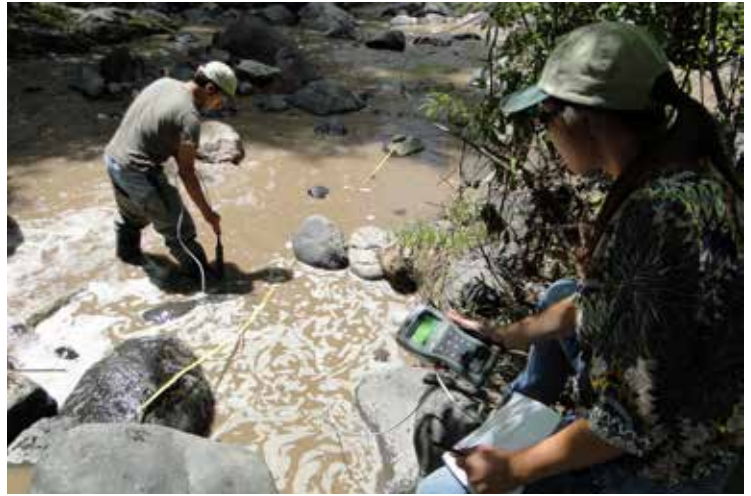
Here, students using the professional-grade Hanna meter for water quality studies, which tests up to 13 parameters of water.
