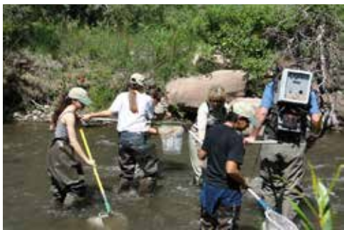
Students use various science equipment at the Institute. Here, the electroshock fish backpack unit, to examine fish and conduct related surveys.
