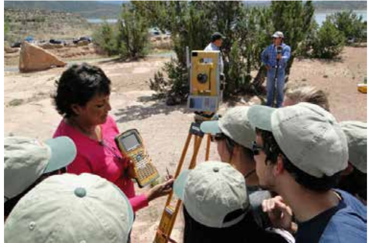
Here, students use the Robotic Field Total Surveying Station with CAD Software, which plots/maps a variety of topographic and ecological data.
